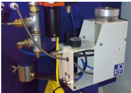
Application of microblast with a mikromat 50 eco
